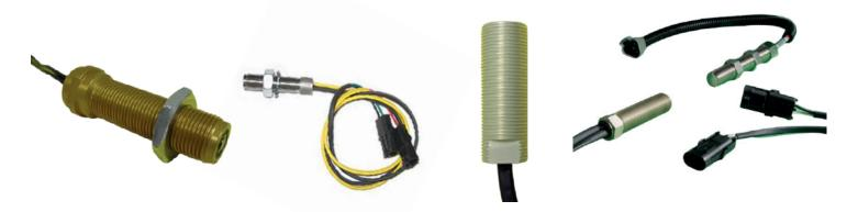
Non-contact magnetic sensors that measure the collapse of magnetic field due to the interruption by a ferrous gear tooth. These sensors provide two analog signal outputs (sine wave) that does not require an outside power source. This sensor is suitable for speed sensing with a range from 30 to 1000 inches per second with a target gear from one tooth per revolution to 32 pitch gear.
